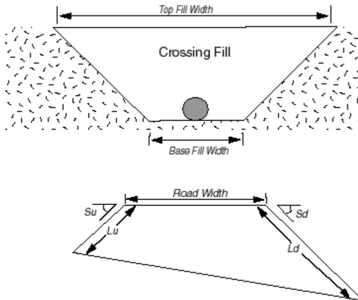
*Crossing fill measurements.* Note that  $L_d$ , the downstream fill slope length often extends below the culvert outlet. These measurements are for obtaining a rough estimate of the fill volume and not intended for use in contract specifications.
