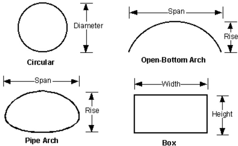
Height- The height, rise, or diameter (measured vertically) of the culvert, measured from the inside of the corrugations. If the culvert bottom is completely covered with bedload (embedded) estimate the culvert height based on the shape (e.g. assume the height = width for circular culverts). For Open-Bottom Arches, measure the height from the streambed to the top of the culvert.
