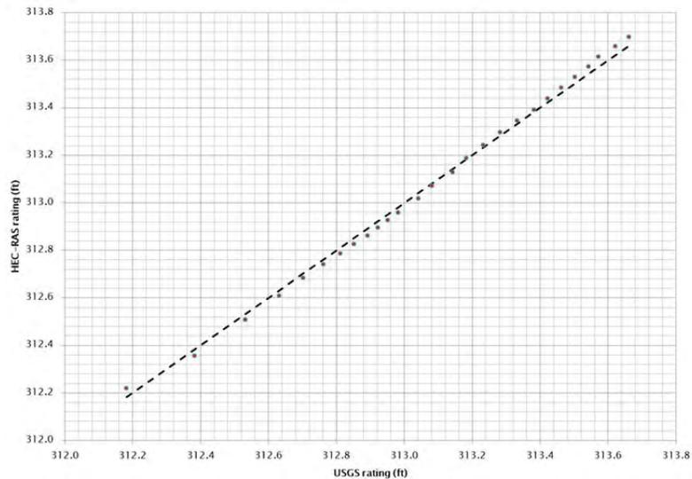
Figure 30. Observed vs. predicted stage-discharge relationships for the Welch Creek gage (USGS #11-173575, Node 4) for steady-state discharges ranging from 1 cfs to 300 cfs. Dashed line represents perfect agreement.
