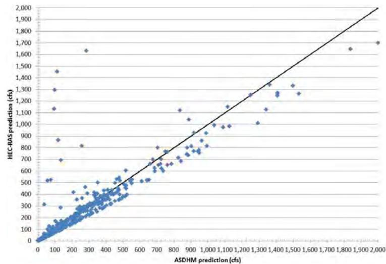
Figure 36. Comparison of HEC-RAS computed flows at Node 4 compared to ASDHM computed flows. Line represents perfect agreement.
