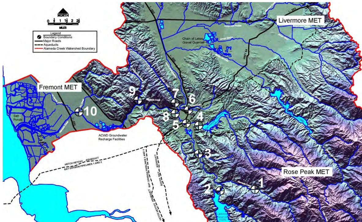
Figure 35. Hydrology and water temperature boundary condition locations for the unsteady HEC-RAS water temperature model, and meteorological stations (MET) used for the water temperature model.
