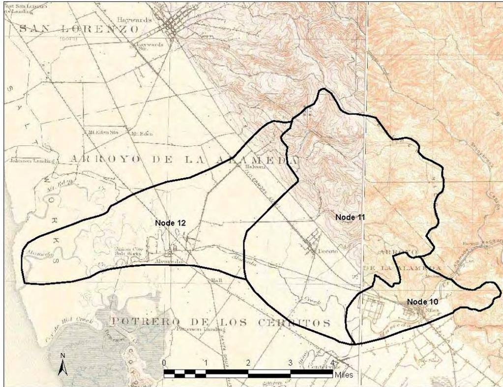
Figure 4. Example of drainage area boundary used in scaling unimpaired gages to ungaged tributaries and watershed areas, using the lower portion of Alameda Creek.
