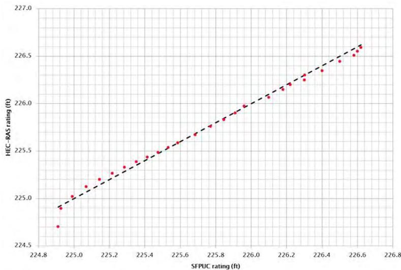
Figure 31. Observed vs. predicted stage-discharge relationships for the SFPUC gaging station at the Water Temple, immediately upstream of the Arroyo de la Laguna confluence (Node 7) for steady-state discharges ranging from 1 cfs to 300 cfs. Dashed line represents perfect agreement.
