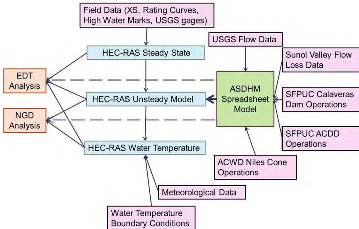
Figure 2. Components of Alameda Creek flow and temperature modeling effort.
