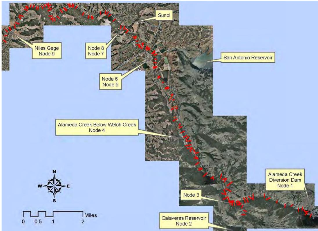
Figure 27. Cross sections used for steady-state and unsteady HEC-RAS model.
