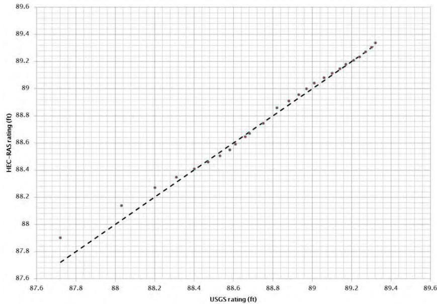
Figure 32. Observed vs. predicted stage-discharge relationships for the Niles gage (USGS #11-179000, Node 9) for steady-state discharges ranging from 1 cfs to 300 cfs. Dashed line represents perfect agreement.
