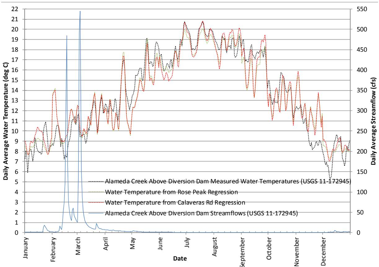
Figure 38. Example comparison of predicted daily average water temperature in 2009 at the Above ACDD gage (USGS #11-172945) using the 3-day average air temperature from two different meteorological stations.
