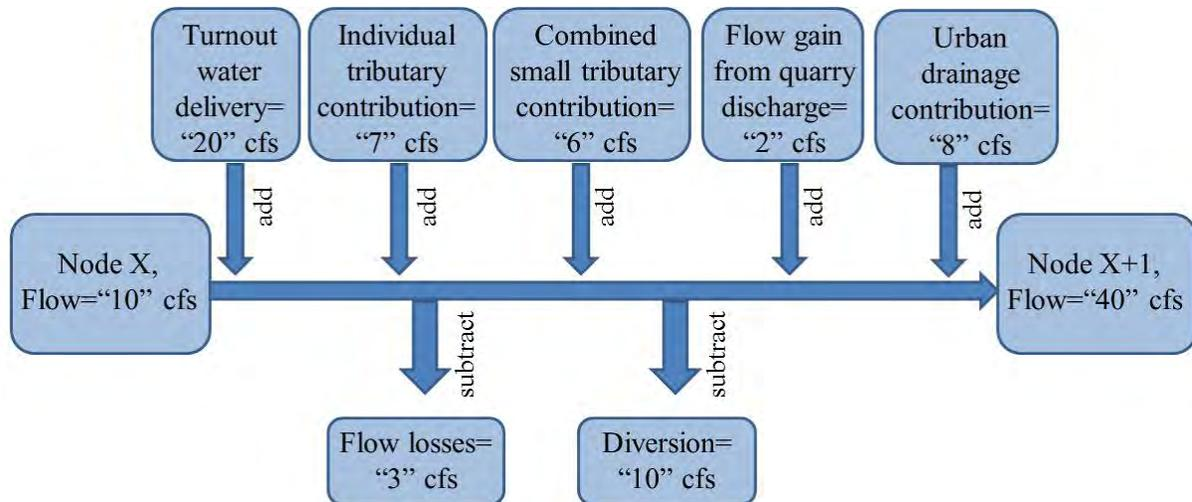
Figure 3. Simplified illustration of computational procedure incorporated in ASDHM.
