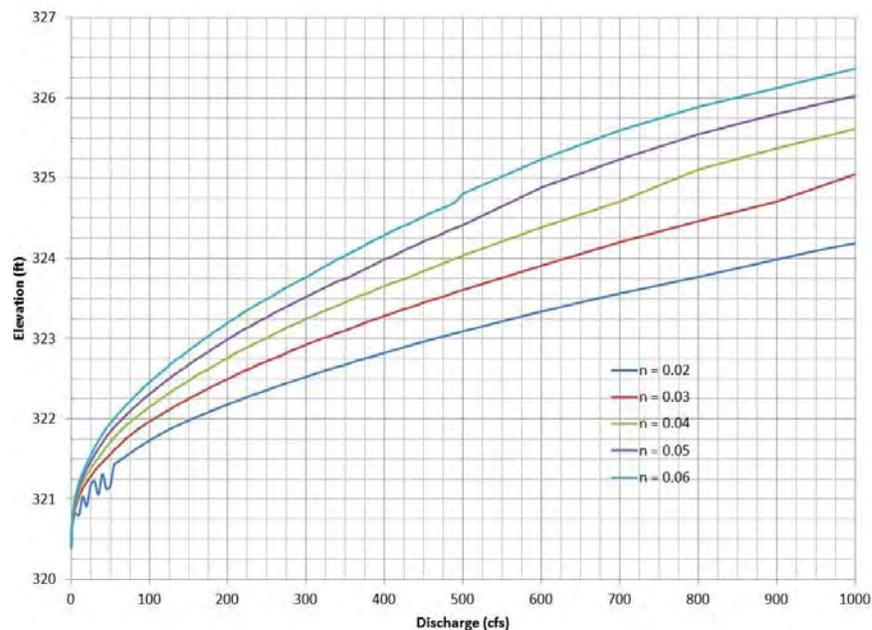
Figure 29. Modeled stage-discharge relationships with varying Manning's  $n$  values using flows from the Welch Creek gage (USGS #11-173575).
