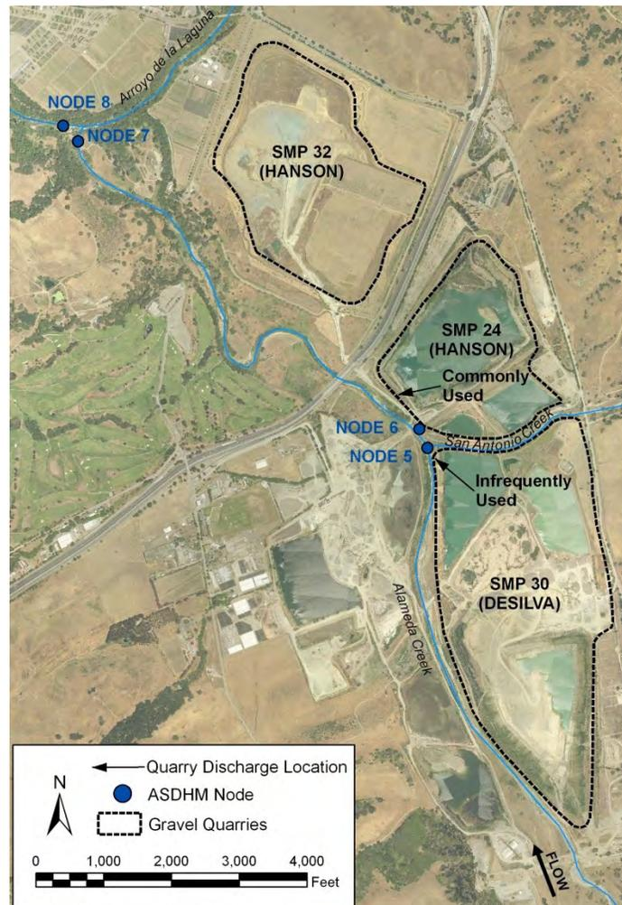
Figure 12. Gravel quarries in lower Sunol Valley and approximate discharge points. There is a cut-off wall on SMP-32, a partial cut-off wall on SMP-24, and no cut-off wall on SMP-30.
