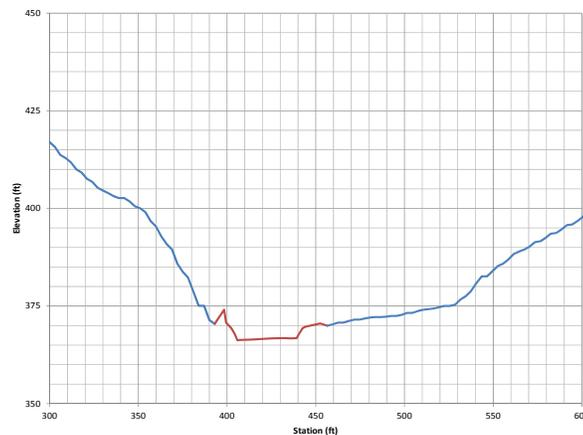
Figure 28. Example integration of field-based cross section surveys (red) with LiDAR based topography (blue) to generate final cross sections for the HEC-RAS model.
