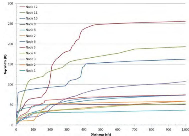
Figure 34. Total channel wetted top width as a function of local flow at each of the 12 nodes.
