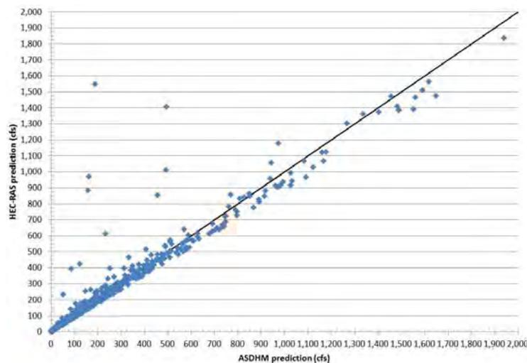
Figure 37. Comparison of HEC-RAS computed flows at Node 7 compared to ASDHM computed flows. Line represents perfect agreement.
