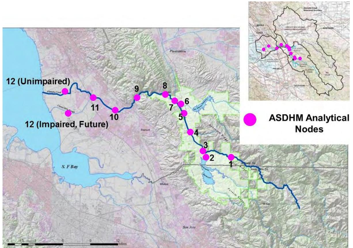
Figure 1. Spatial extent of hydrology, hydraulic, and water temperature modeling efforts, and ASDHM analytical nodes where flow computations are summarized by the various scenarios.
