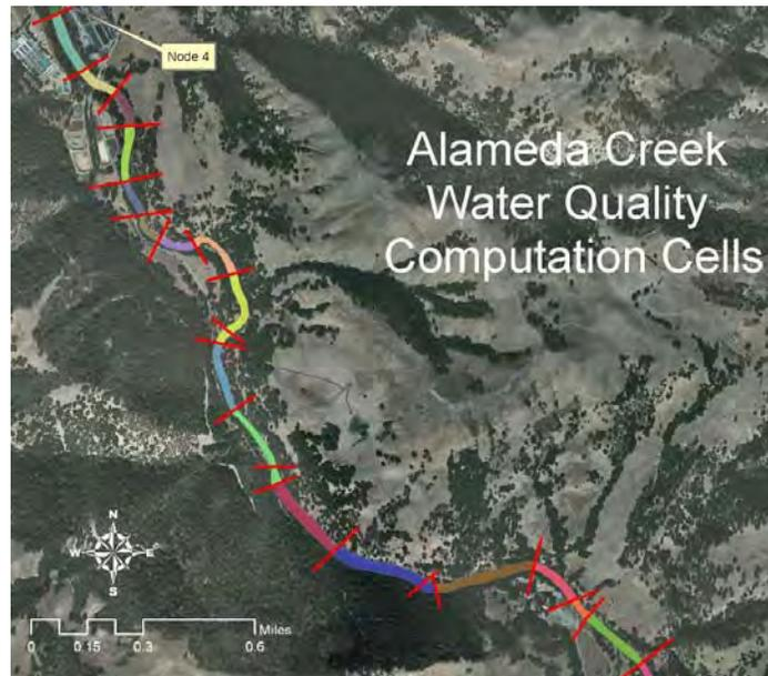
Figure 42. HEC-RAS water temperature model computational cells upstream of Node 4.
