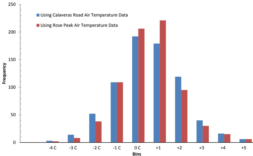
Figure 39. Example evaluation of bias between the two different meteorological stations considered for predicting water temperature boundary conditions at the Above ACDD gage location (USGS #11-173945, Node 1). In this example, the Calaveras Road meteorological station was chosen over the Rose Peak station.
