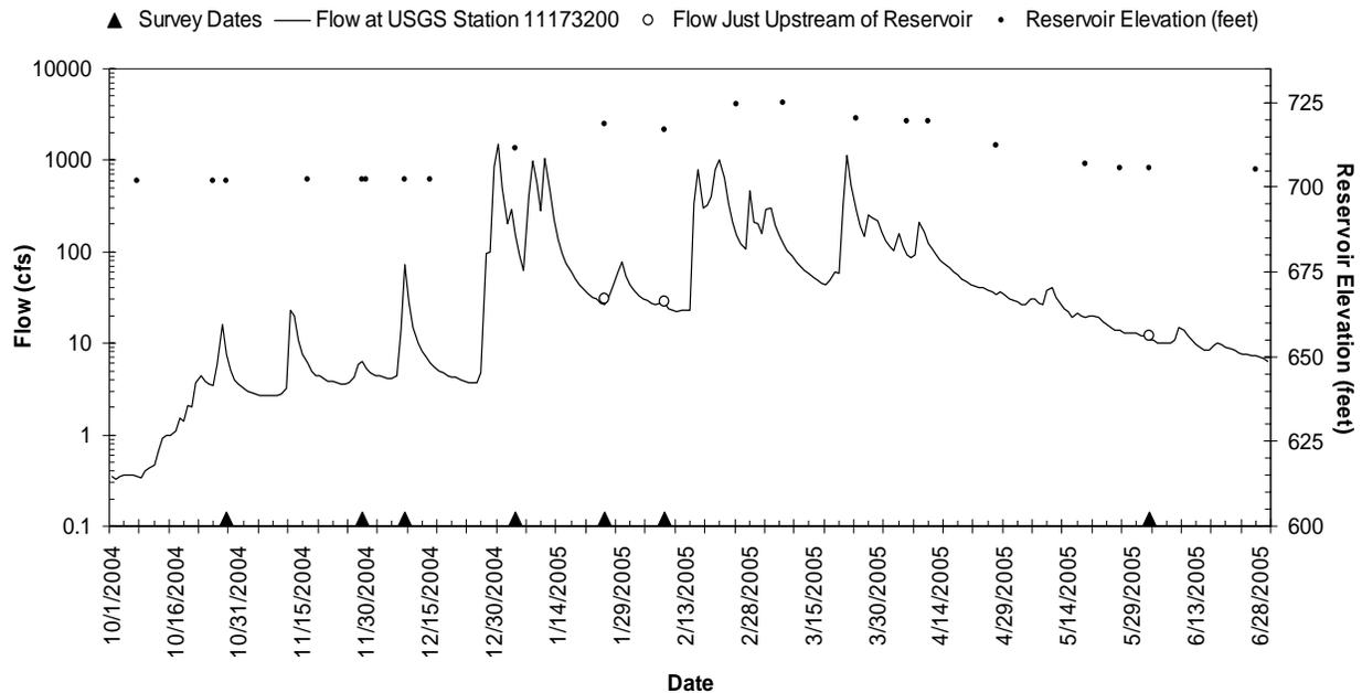
**Figure 4.** *Arroyo Hondo surface flows at USGS gauging station 11173200 near Marsh Road, flows just upstream of Calaveras Reservoir and reservoir elevations.*
