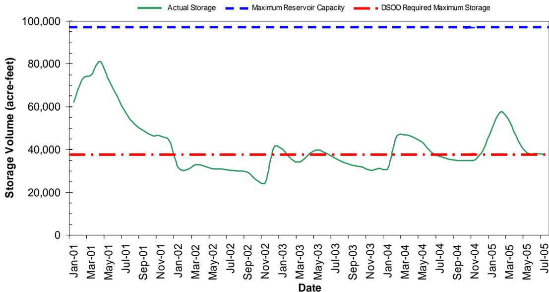
**Figure 1.** Average monthly storage at Calaveras Reservoir, with the maximum reservoir capacity and the DSOD requirement equivalent superimposed.
