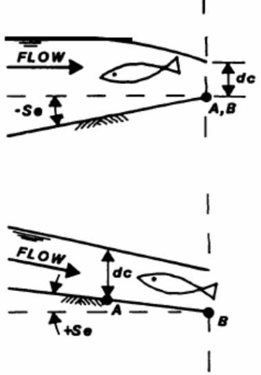
8. Is critical depth (dc) located too far upstream for fish to reach during landing?
