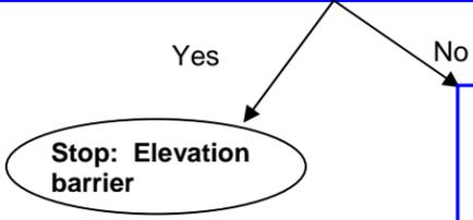
2. Is the horizontal distance from the crest of the falls to the standing wave (X) greater than the horizontal distance of the fish's leap at the highest point of the leap (XL)?
