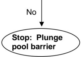
5. Is the length of the fish (LF) greater than the depth of the plunge pool (dpp)?
